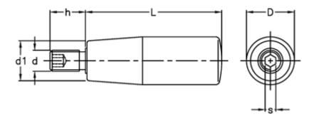
$$\begin{array}{ll} D & = 23 \\ d1 & = 19 \\ d 6g = M8 \\ h & = 15 \\ L & = 65 \\ s & = 4 \end{array}$$
